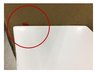
Fold the protective film of double-sided tape to the out side in advance as shown in the figure. This allows you to easily pull out the protective film and fixed the side skirt to the body.
