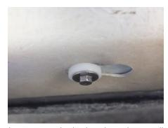
Pass the stud pin through the hole of the resinous washer. Then push up the side skirt against the body side and reinstall the stud pin to the body side together with resinous washer. As shown in the figure.
