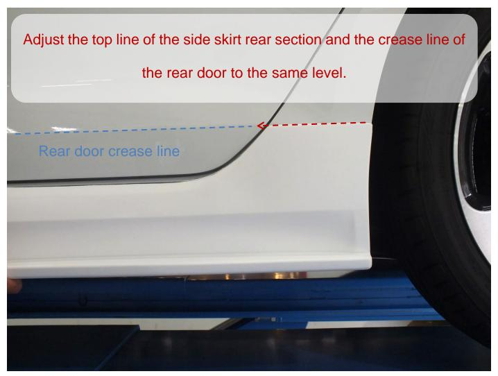
Keep the correct mounting position (Adjust the top line of the side skirt rear section and the crease line of the rear door to the same level)
